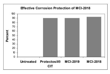
As the graph indicates, MCI-2018 provides >92% protection from corrosion when compared to untreated concrete and outperforms the competitive products.
