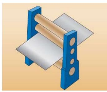
To provide the cleanest strip possible, most material is wet rolled at the temper mill. For rolled steel, VpCI-344 diluted with water can be used as a wet tempering fluid.
